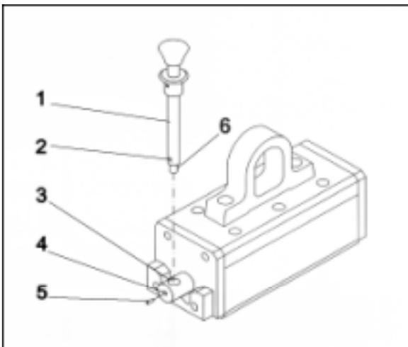
**Attention!** Ensure that the end of the stud (5) fully engages in the notch (2) of the handle and secures it in place. Check that the locking shaft (6) protrudes from the shaft as shown and blocks the handle from accidental rotation.
